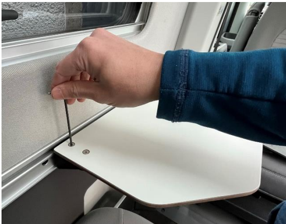
Figure 3. When the table is at the desired angle tighten the four countersunk socket screws.
